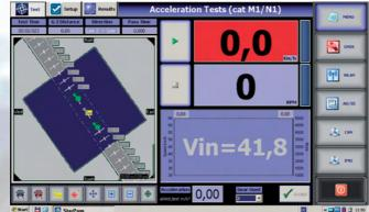
uses both the code and phase signals to determine the vehicle position (carrier Phase Doppler technique), while the speed calculation is refined via a Von Kalmann filter optimized for dynamic performance.
